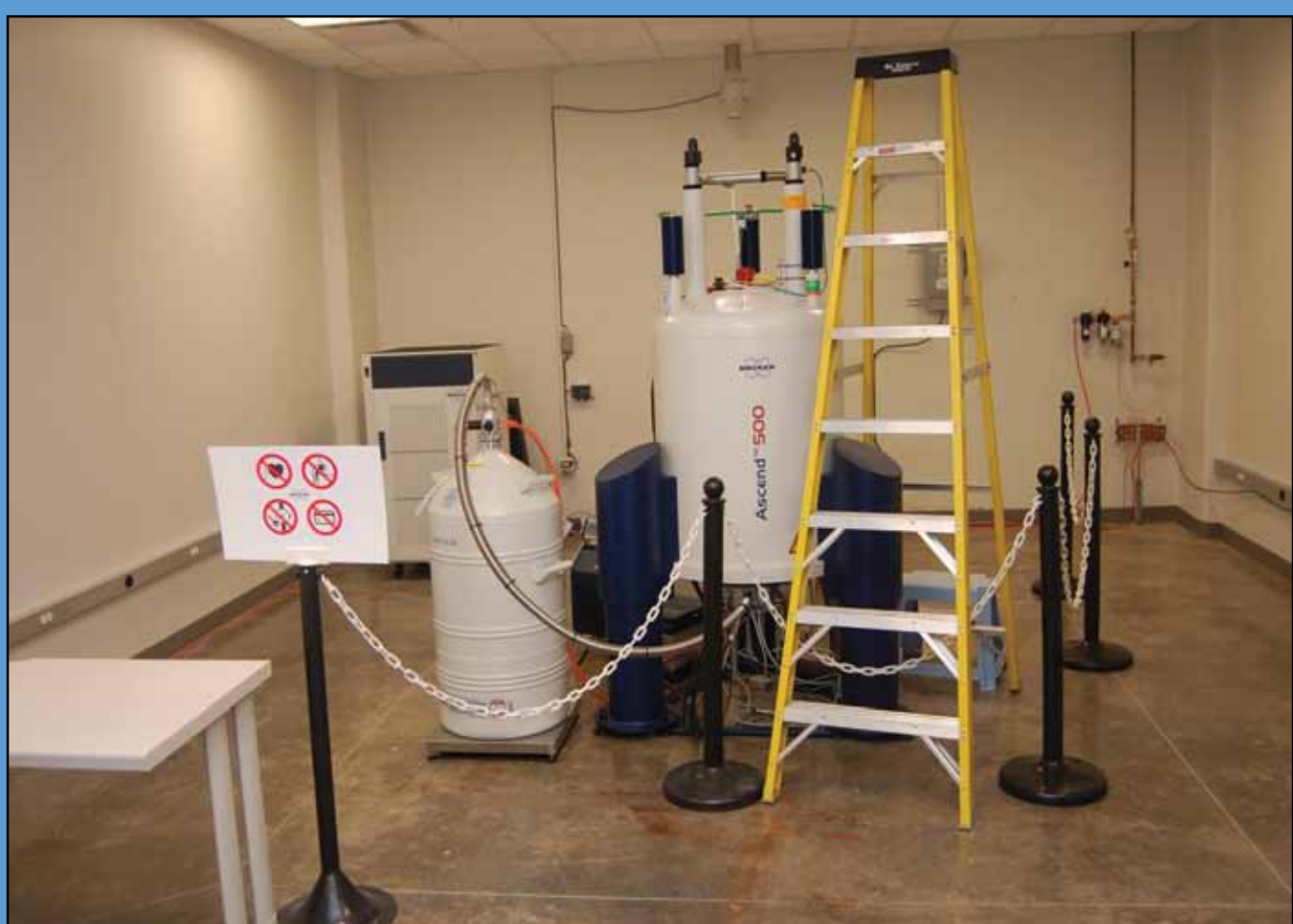
Figure 4. NMR system Bruker AV-III-500HD 2
