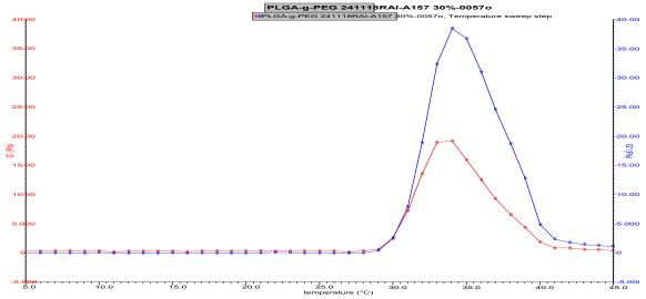
**Rheology** performed on AR2000 (TA instruments) with 60mm 2degree cone on 30% w/v polymer in PBS dissolved over 24 hours with stirring at 4°C. Viscosity of solution at 0.1 (sec<sup>-1</sup>) and 5°C was measured (1 minute peak hold 5 second test intervals). Rheology performed by oscillating at constant 6.283 rad/s, 0.1% strain, in increments of 1°C ranging from 5-45°C with 1 minutes of temperature equilibration at each point.
