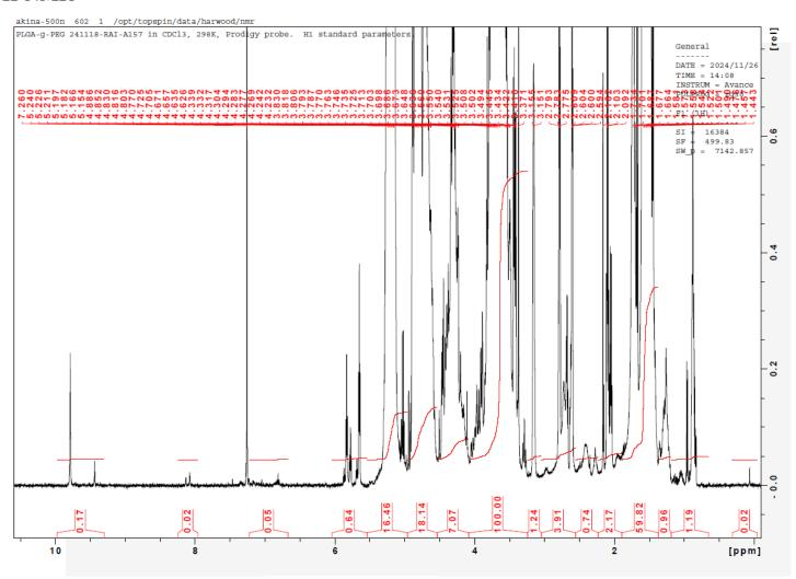
**H-NMR** Spectrum of copolymers in CDCl3 (Bruker ≥300 MHz, PINMRF) NMR of PLGA-g-PEG copolymer: LA:GA:EG = 1.8 : 1 : 2.7
