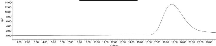
**GPC Analysis Method:** Waters Breeze 2 system with 1 ml/min THF flow across three GPC columns. Detection via refractive index, calibrated against polystyrene standards (Agilent Polystyrene, PS2).
