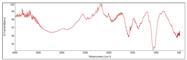
FTIR Analysis: Collected from IS5 ID7-ATR spectrometer (Thermo Scientific) and analyzed in transmission mode.
