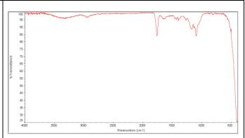
FTIR Analysis: Collected from cast-film on KBr salt-plate placed in Nicollet Avatar 320 spectrometer and analyzed in transmission mode.
