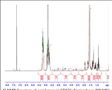
H-NMR Spectrum of copolymers in CDC13 (Varian Inova 500 MHz instrument) NMR of PLGA copolymer: LA-GA =50%/50% molar
