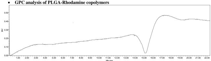
Analysis Method: Waters Breeze 2 system with 1 ml/min DCM flow across three GPC columns (7.8 x 300 mm, mixed porosities). Detection via refractive index, calibrated against polystyrene standards.
