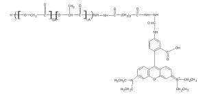
**Dye Content:** Testing of absorbance of polymer in DCM solution at 543 nm as compared to series of RITC standards has indicated a dye content of:  $5.9 \mu g/mg$  polymer.
