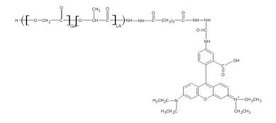
**Dye Content:** Testing of absorbance of polymer in DCM solution at 543 nm as compared to series of Rhodamine-B isothiocyanate standards has indicated a dye content of: 26.34 μg/mg polymer.
