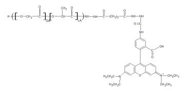
**Dye Content:** Testing of absorbance of polymer in DCM solution at 543 nm as compared to series of RITC standards has indicated a dye content of: 9.09 µg/mg polymer.
