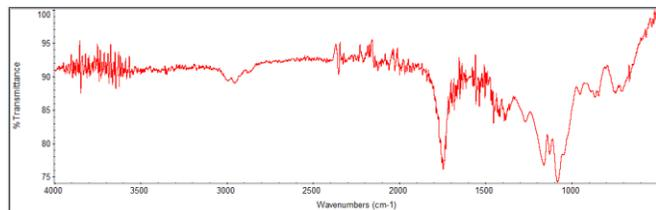
FTIR Analysis: Collected from Nicolet Avatar 380 spectrometer with ATR Smart Orbit and analyzed in transmission mode.
