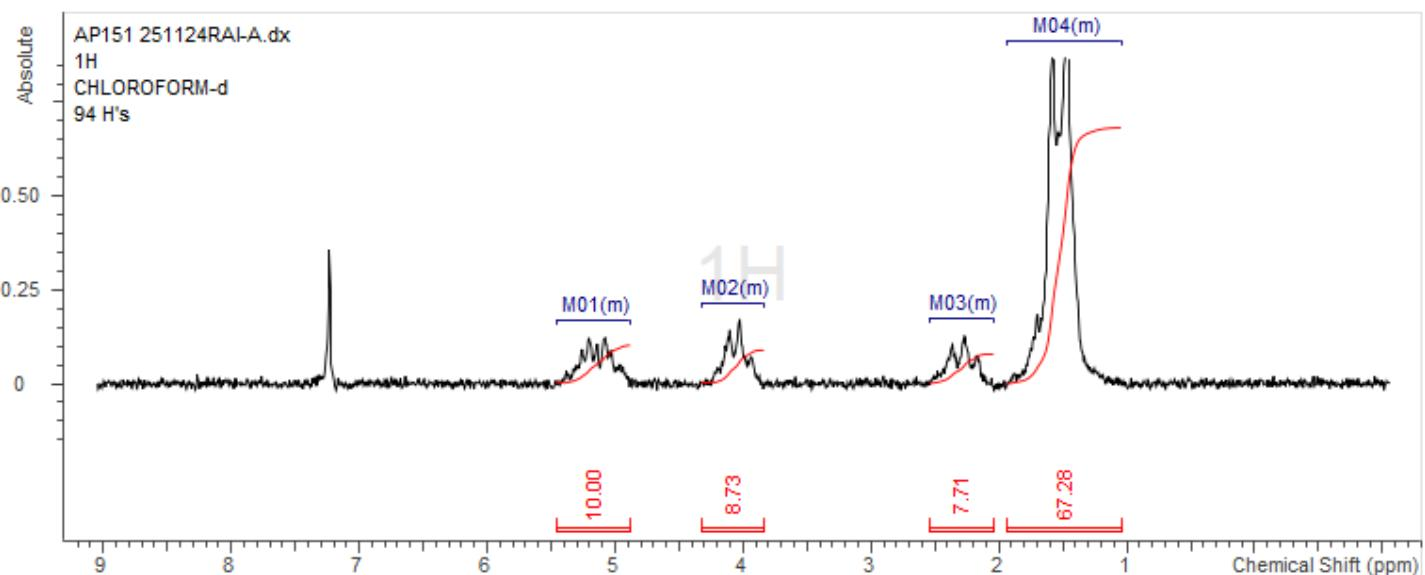
**H-NMR** Spectrum of copolymers in CDCl<sub>3</sub> (NMReady-60e, Nanalysis 60 MHz) NMR of PDLCL copolymer: LA-CL =70%-30% molar ratio (LA:CL 74%:26% w:w)
