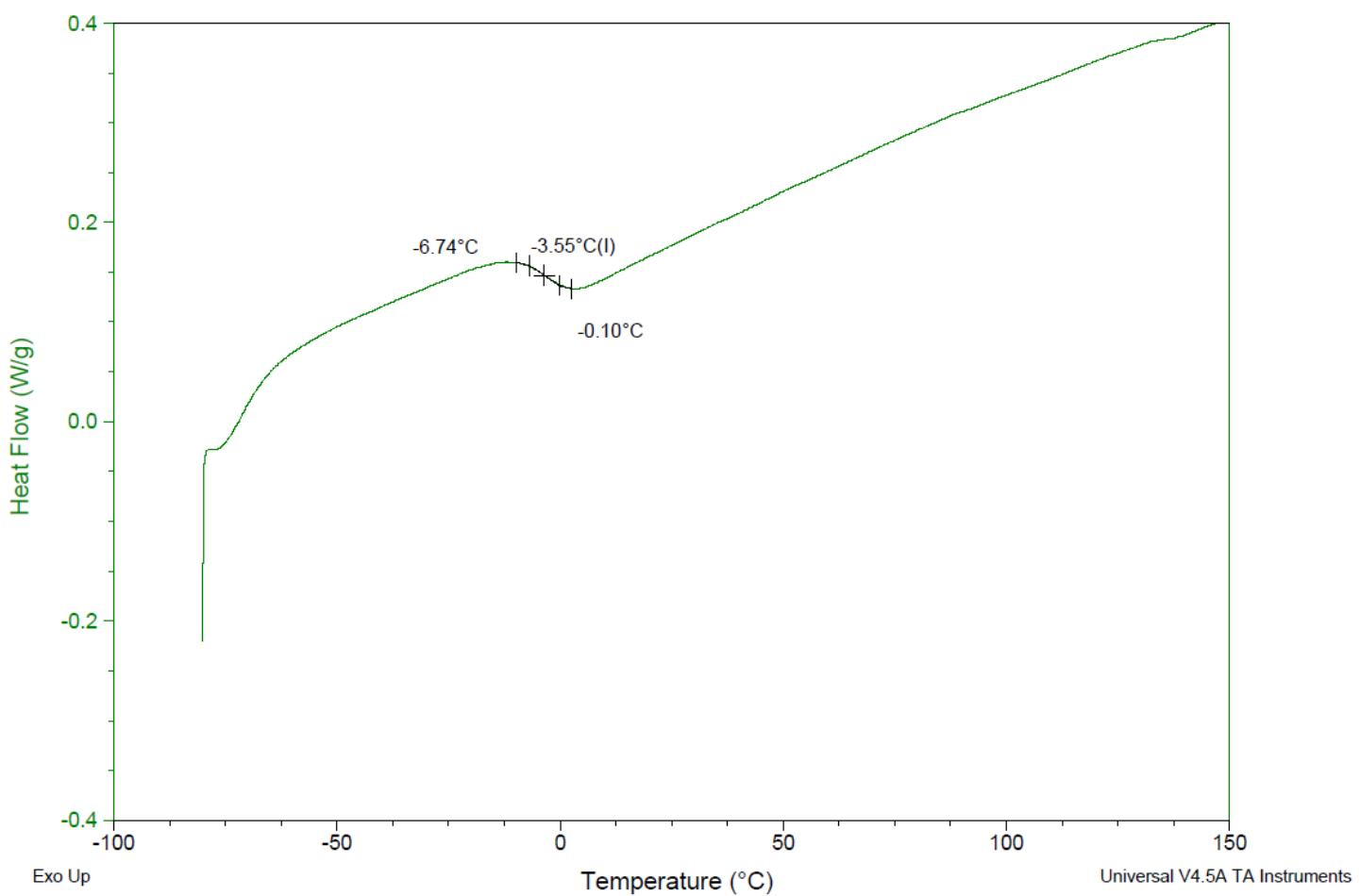
**DSC Testing:** 1-5 mg sample tested in crimped aluminum pan on a TA Instruments Model Q2000 with procedure equilibration 100 °C, isothermal 5 minutes, equilibrate -80 °C, data on, ramp 10 °C/min to 150 °C.  $T_g = -3.55$  °C
