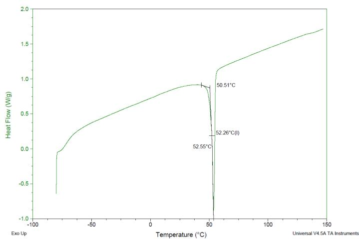
**DSC** Testing: 1-5 mg sample tested in crimped aluminum pan on a TA Instruments Model Q2000 with procedure equilibraion 100 °C, isothermal 5 minutes, equilibrate -80 °C, data on, ramp 10 °C/min to 150 °C. Tg = 52.26 °C
