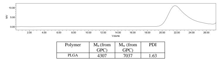
GPC-ES Analysis Method: Waters Breeze 2 system with 1 ml/min THF flow across three GPC columns. Detection via refractive index, calibrated against polystyrene standards.
