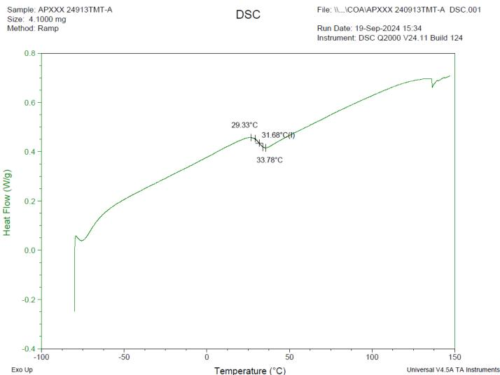
DSC Testing: 1-5 mg sample tested in crimped aluminum pan on a TA Instruments Model Q2000 with procedure equilibraion 100 °C, isothermal 5 minutes, equilibrate -80 °C, data on, ramp 10 °C/min to 150 °C. Tg = 31.68 °C
