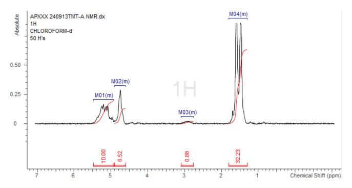
H-NMR Spectrum of copolymers in CDCl3 (Bruker ≥300 MHz, PINMRF) NMR of PLGA copolymer: LA-GA =75%-25% molar ratio (LA:GA 79%:21% w:w)
