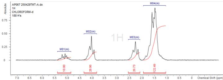
H-NMR Spectrum of copolymers in CDCl3 (NMReady-60e, Nanalysis 60 MHz) NMR of P(L)LCL copolymer: LA-CL =41%:59% molar ratio (LA:CL 30%:70%)
