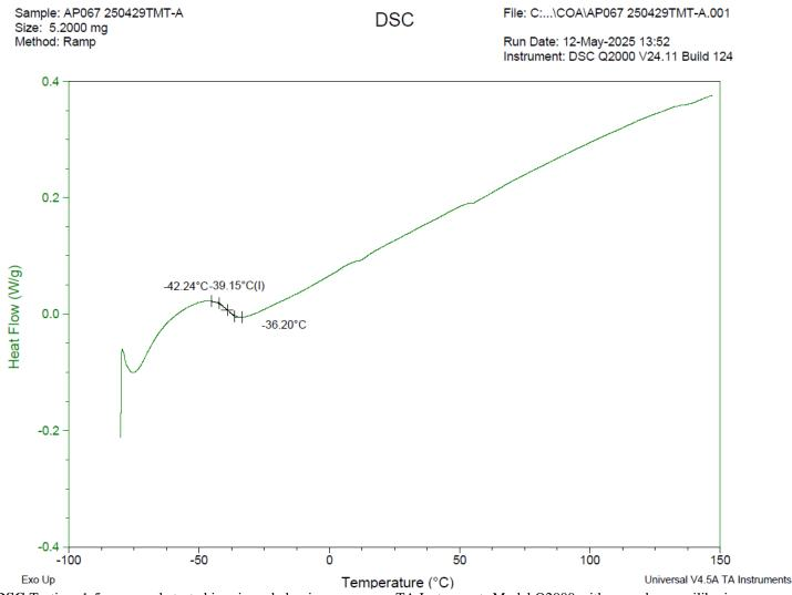
**DSC** Testing: 1-5 mg sample tested in crimped aluminum pan on a TA Instruments Model Q2000 with procedure equilibration 100 °C, isothermal 5 minutes, equilibrate -80 °C, data on, ramp 10 °C/min to 150 °C. Tg = 39.15 °C
