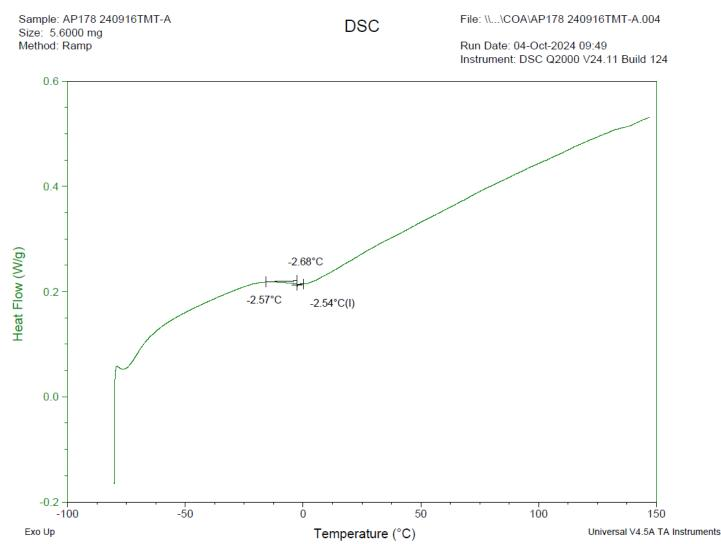
DSC Testing: 1-5 mg sample tested in crimped aluminum pan on a TA Instruments Model Q2000 with procedure equilibration 100 °C, isothermal 5 minutes, equilibrate -80 °C, data on, ramp 10 °C/min to 150 °C. Tg = -2.54 °C
