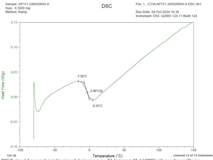
DSC Testing: 1-5 mg sample tested in crimped aluminum pan on a TA Instruments Model Q2000 with procedure equilibration 100 °C, isothermal 5 minutes, equilibrate -80 °C, data on, ramp 10 °C/min to 150 °C. Tg = -2.90 °C
