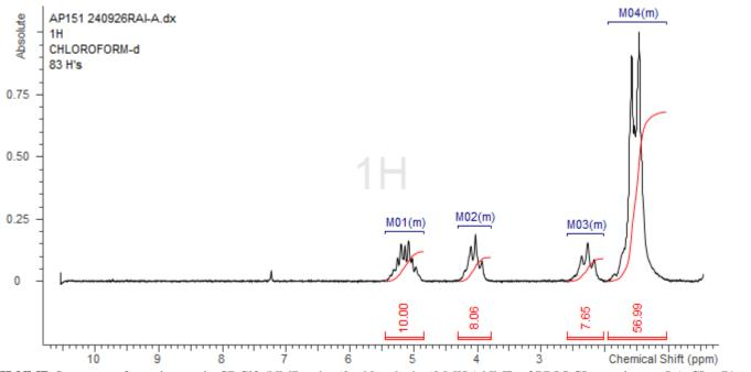
**H-NMR** Spectrum of copolymers in CDCl3 (NMReady-60e, Nanalysis 60 MHz) NMR of PDLLCL copolymer: LA-CL =71%-29% molar ratio (LA:CL 61%:39% w"w)
