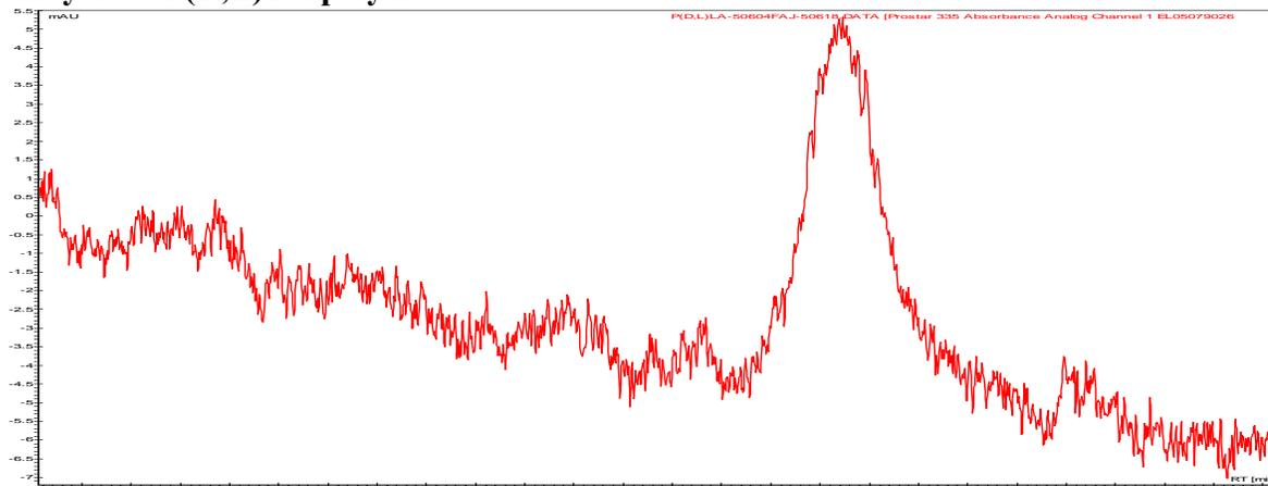
Analysis Method: Varian Prostar system with 1 ml/min DCM flow across two PLgel mixed-D columns and one Mixed-E column (Agilent). Detection via UV/Vis, calibrated against polystyrene standards
