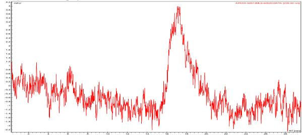
Analysis Method: Varian Prostar system with 1 ml/min DCM flow across two PLGel Resipore columns (Agilent). Detection via UV/Vis, calibrated against polystyrene standards.
