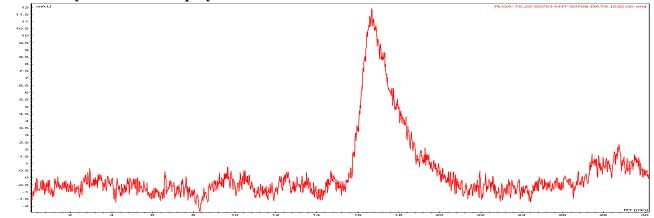
Analysis Method: Varian Prostar system with 1 ml/min DCM flow across three Phenogel columns and one PLgel Resipore column (Agilent). Detection via UV/Vis, calibrated against polystyrene standards
