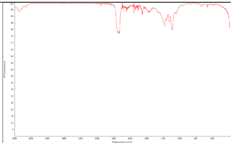
FTIR Analysis Method: Collected from cast-film on salt-plate placed in Protégé 460 Spectrometer (Nicolet) and analyzed in Transmission E.S.P. mode
