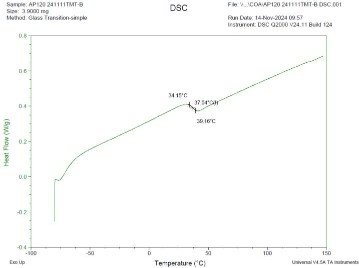
**DSC** Testing: 1-5 mg sample tested in crimped aluminum pan on a TA Instruments Model Q2000 with procedure equilibration 100 °C, isothermal 5 minutes, equilibrate -80 °C, data on, ramp 10 °C/min to 150 °C. Tg = 37.04 °C
