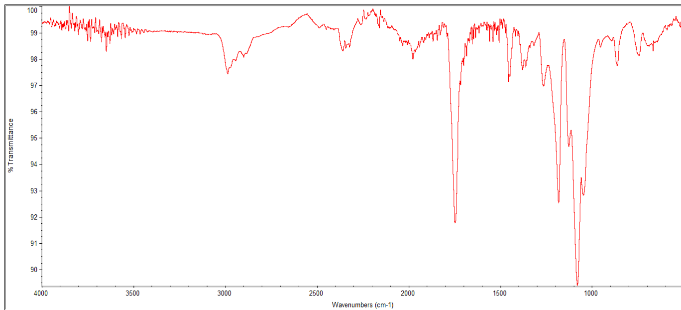
FTIR Analysis: Collected from IS5 ID7-ATR spectrometer (Thermo Scientific) and analyzed in transmission mode.
