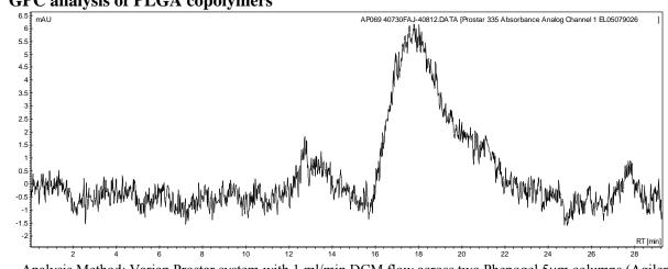
Analysis Method: Varian Prostar system with 1 ml/min DCM flow across two Phenogel 5µm columns (Agilent). Detection via UV/Vis, calibrated against polystyrene standards.
