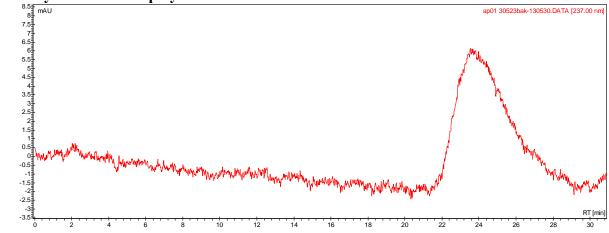
Analysis Method: Varian Prostar system with 1 ml/min DCM flow across three Phenogel 5u columns and one PLgel Resipore columns (Agilent). Detection via UV/Vis, calibrated against polystyrene standards
