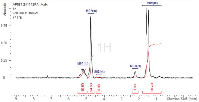
**H-NMR** Spectrum of copolymers in CDCl3 (NMReady-60e, Nanalysis 60 MHz) NMR of PLGA copolymer: LA-GA =45%-55% molar ratio (LA:GA 50%:50% w:w Da)
