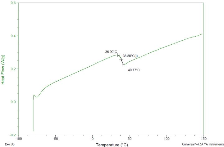
**DSC** Testing: 1-5 mg sample tested in crimped aluminum pan on a TA Instruments Model Q2000 with procedure equilibraion 100 °C, isothermal 5 minutes, equilibrate -80 °C, data on, ramp 10 °C/min to 150 °C. Tg = 38.8 °C
