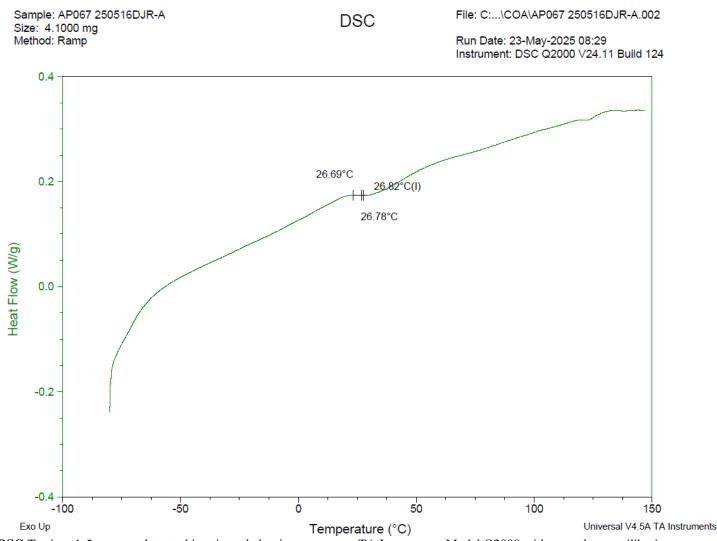
**DSC** Testing: 1-5 mg sample tested in crimped aluminum pan on a TA Instruments Model Q2000 with procedure equilibration 100 °C, isothermal 5 minutes, equilibrate -80 °C, data on, ramp 10 °C/min to 150 °C. Tg = 26.82 °C
