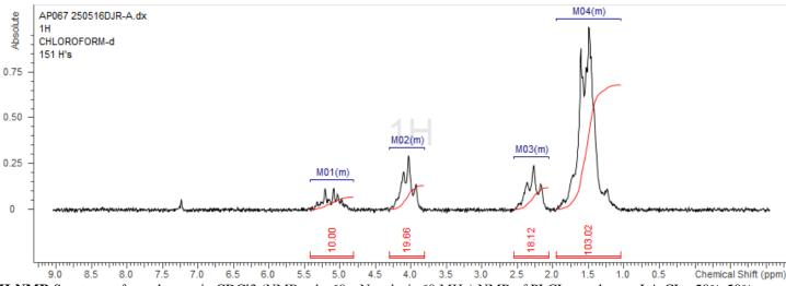
H-NMR Spectrum of copolymers in CDCl3 (NMReady-60e, Nanalysis 60 MHz) NMR of PLCL copolymer: LA-CL =50%-50% molar ratio (LA:GA 56%:44% w:w)
