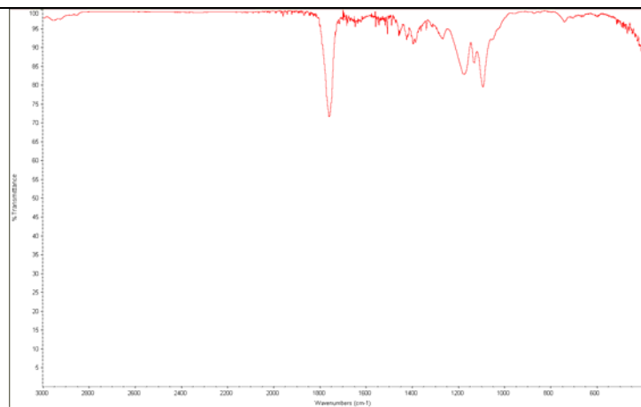
FTIR Analysis Method: Collected from cast-film on KBR salt-plate placed in Protégé 460 Spectrometer E.S.P. (Nicolet) and analyzed in Transmission E.S.P. mode.
