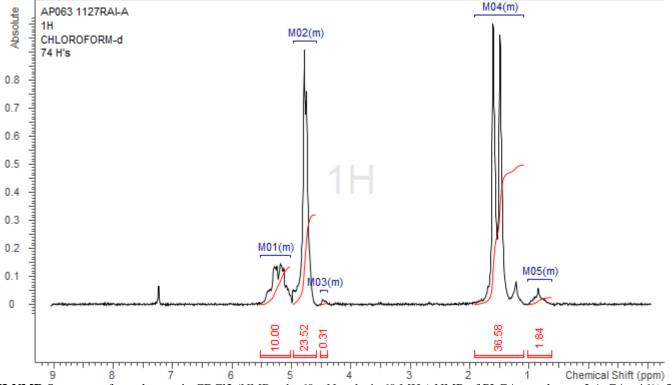
**H-NMR** Spectrum of copolymers in CDCl3 (NMReady-60e, Nanalysis 60 MHz) NMR of PLGA copolymer: LA-GA =46%:54% molar ratio (LA:GA 51%:49% Da)
