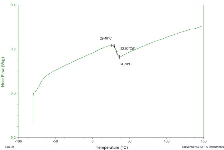
**DSC** Testing: 1-5 mg sample tested in crimped aluminum pan on a TA Instruments Model Q2000 with procedure equilibraion 100 °C, isothermal 5 minutes, equilibrate -80 °C, data on, ramp 10 °C/min to 150 °C. Tg = 32.60 °C
