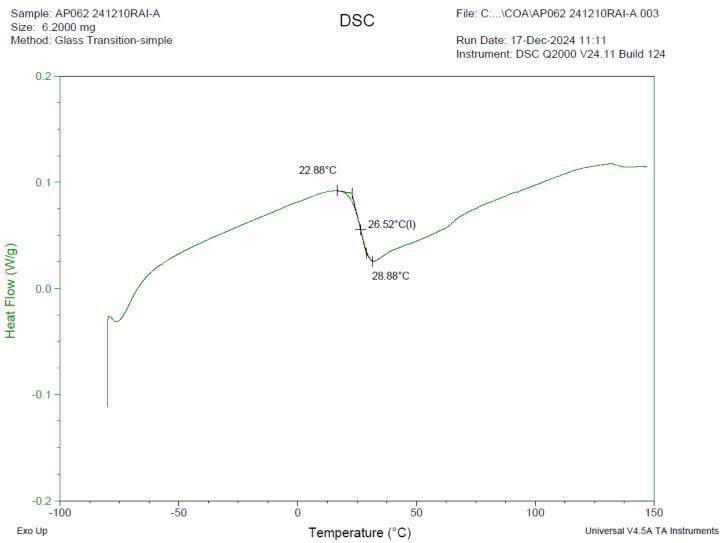
**DSC** Testing: 1-5 mg sample tested in crimped aluminum pan on a TA Instruments Model Q2000 with procedure equilibraion 100 °C, isothermal 5 minutes, equilibrate -80 °C, data on, ramp 10 °C/min to 150 °C. Tg = 26.52 °C
