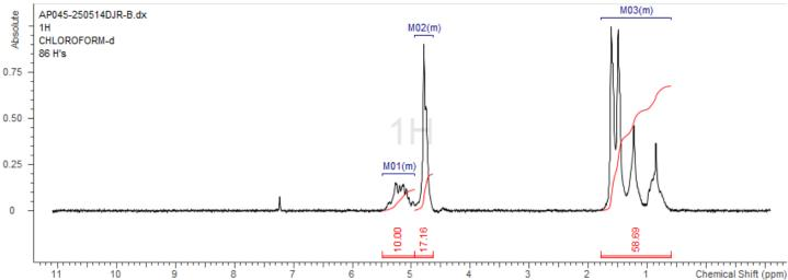
**H-NMR** Spectrum of copolymers in CDCl3 (NMReady-60e, Nanalysis 60 MHz) NMR of PLGA copolymer: LA-GA =54%-46% molar ratio (LA:GA 59%:41% w:w)
