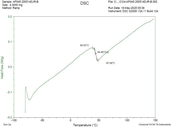
**DSC** Testing: 1-5 mg sample tested in crimped aluminum pan on a TA Instruments Model Q2000 with procedure equilibraion 100 °C, isothermal 5 minutes, equilibrate -80 °C, data on, ramp 10 °C/min to 150 °C. Tg = 44.46 °C
