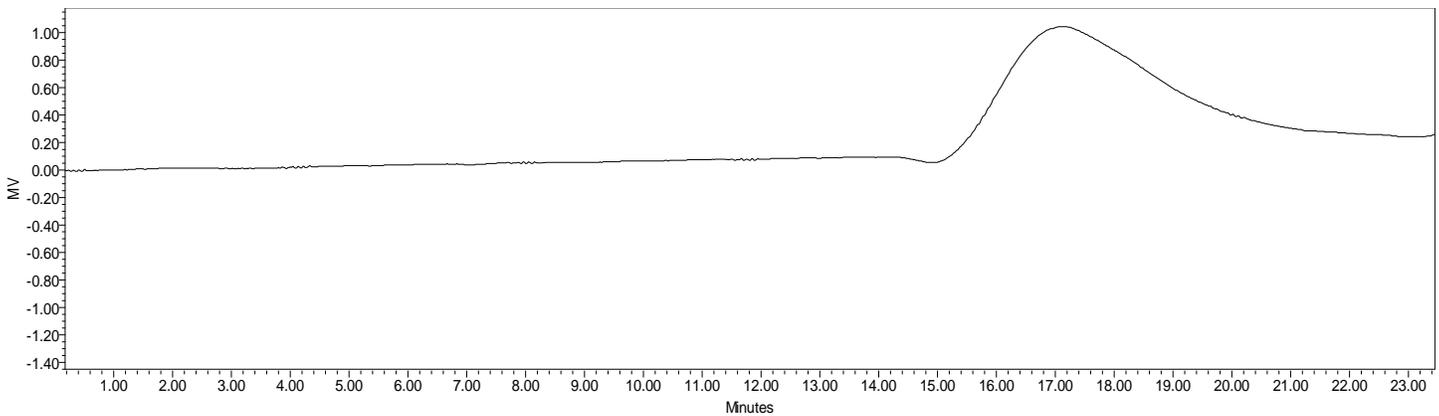
Analysis Method: Waters Breeze 2 system with 1 ml/min DCM flow across three Phenogel 5um columns (Phenomenex). Detection via refractive index, calibrated against polystyrene standards.
