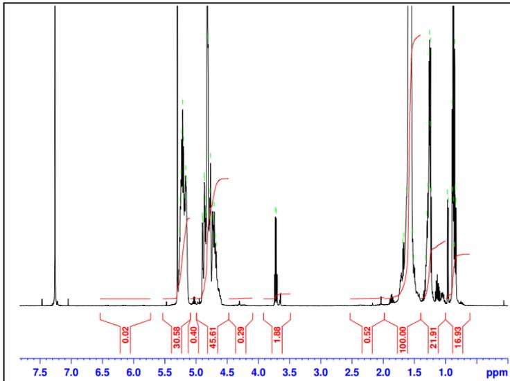
H-NMR Spectrum of PLGA copolymer in CDCl<sub>3</sub> (Varian Inova 500 MHz instrument), NMR of PLGA copolymers:
