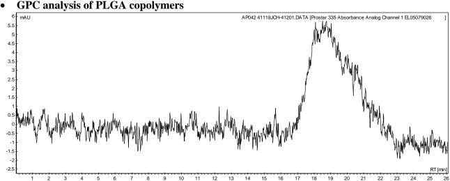
Analysis Method: Varian Prostar system with 1 ml/min DCM flow across two Phenogel 5µm columns and one PLgel Resipore column (Agilent). Detection via UV/Vis, calibrated against polystyrene standards.
