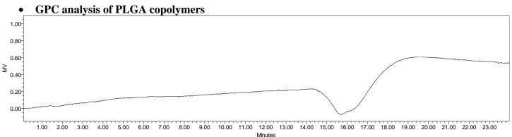
Analysis Method: Waters Breeze 2 system with 1 ml/min DCM flow across two Phenogel 5 µm columns and one PLGel Resipore column (Agilent). Detection via UV/Vis, calibrated against polystyrene standards.
