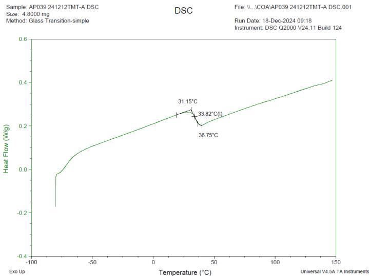
**DSC** Testing: 1-5 mg sample tested in crimped aluminum pan on a TA Instruments Model Q2000 with procedure equilibraion 100 °C, isothermal 5 minutes, equilibrate -80 °C, data on, ramp 10 °C/min to 150 °C. Tg = 33.82 °C
