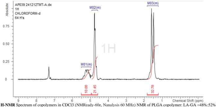
H-NMR Spectrum of copolymers in CDCl3 (NMReady-60e, Nanalysis 60 MHz) NMR of PLGA copolymer: LA-GA molar ratio (LA:GA 54%:46% w:w)
