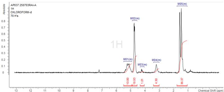
**H-NMR** Spectrum of copolymers in CDCl3 (NMReady-60e, Nanalysis 60 MHz) NMR of PLGA copolymer: LA-GA =51%-49% molar ratio (LA:GA 57%:43% w:w)
