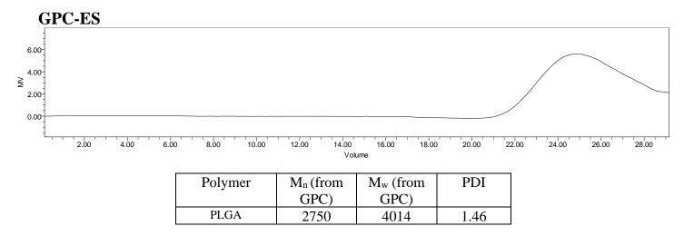
GPC-ES Analysis Method: Waters Breeze 2 system with 1 ml/min THF flow across three GPC columns. Detection via refractive index, calibrated against polystyrene standards.
