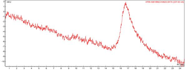
Analysis Method: Varian Prostar system with 1 ml/min DCM flow across two 5µm Phenogel columns and one Resipore column (Agilent). Detection via UV/Vis, calibrated against polystyrene standards.
