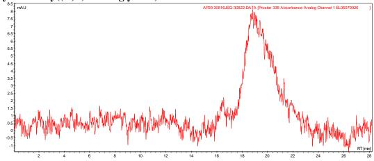
Analysis Method: Varian Prostar system with 1 ml/min DCM flow across two Phenogel 5µ columns and one Resipore column (Agilent). Detection via UV/Vis, calibrated against polystyrene standards.
