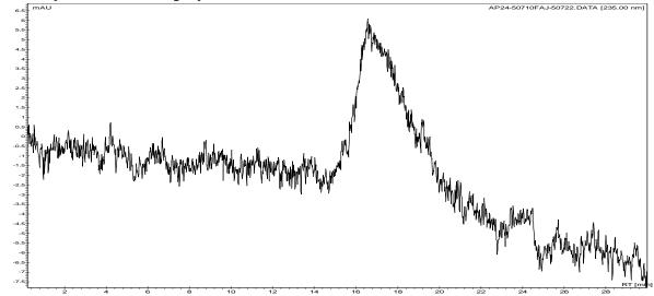
Analysis Method: Varian Prostar system with 1 ml/min DCM flow across two Phenogel 5µm columns and one Resipore column (Agilent). Detection via UV/Vis, calibrated against polystyrene standards.
