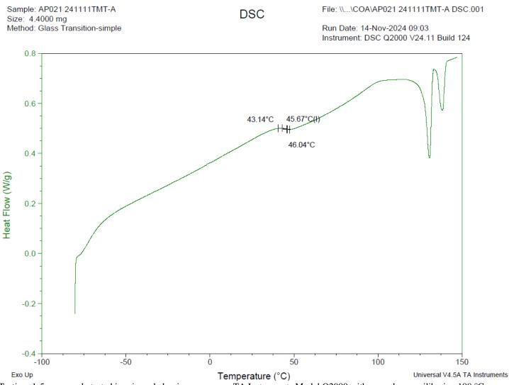
Testing: 1-5 mg sample tested in crimped aluminum pan on a TA Instruments Model Q2000 with procedure equilibraion 100 °C, isothermal 5 minutes, equilibrate -80 °C, data on, ramp 10 °C/min to 150 °C. Tg = 45.67 °C
