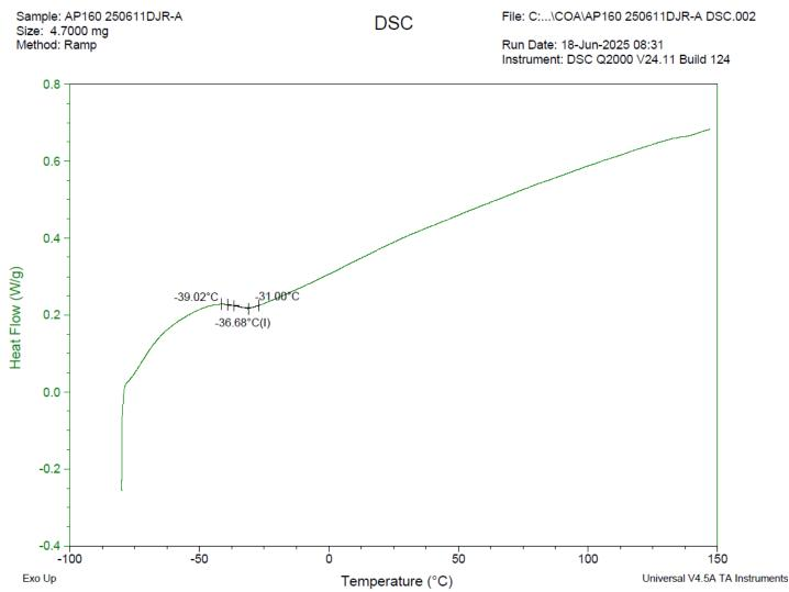
DSC Testing: 1-5 mg sample tested in crimped aluminum pan on a TA Instruments Model Q2000 with procedure equilibraion 100 °C, isothermal 5 minutes, equilibrate -80 °C, data on, ramp 10 °C/min to 150 °C. Tg = -36.68 °C
