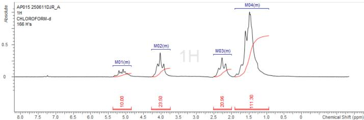
H-NMR Spectrum of copolymers in CDCl3 (NMReady-60e, Nanalysis 60 MHz) NMR of PLLCL copolymer: LA-CL =46%-54% molar ratio (LA:CL 35%:65% w:w)
