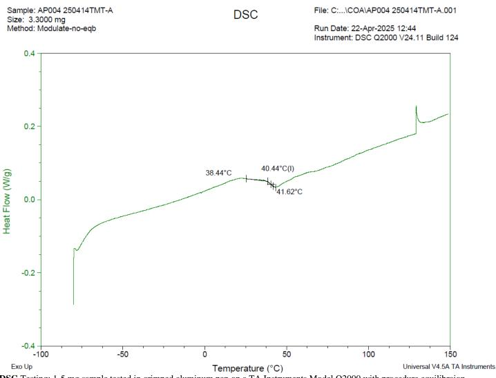
**DSC** Testing: 1-5 mg sample tested in crimped aluminum pan on a TA Instruments Model Q2000 with procedure equilibration 100 °C, isothermal 5 minutes, equilibrate -80 °C, data on, ramp 10 °C/min to 150 °C. Tg = 40.44 °C
