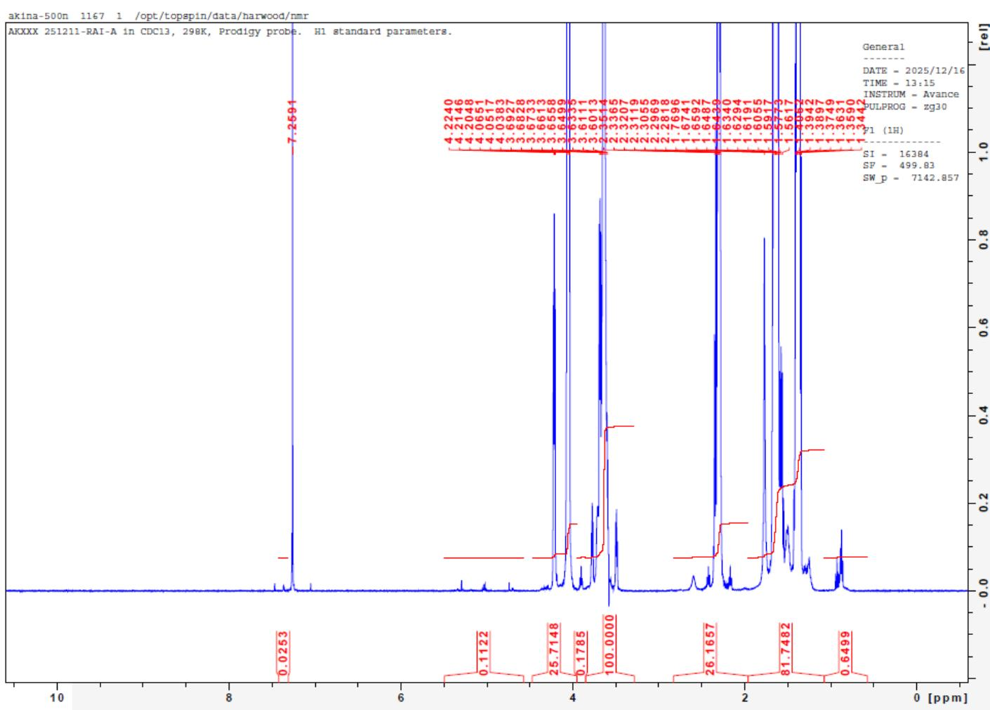
**H-NMR** Spectrum of copolymers in CDCl<sub>3</sub> (Bruker ≥300 MHz, PINMRF) NMR of PCL-PEG-PCL copolymer: EG/CL =33\*/17 (M<sub>n</sub> EG/CL 1454\*/1937 Da) \*- from MFG data
