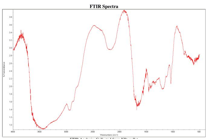
FTIR Analysis: Collected from KBr pellet placed in Protégé 460 Spectrometer (Nicolet) and analyzed in transmission E.S.P. mode.
