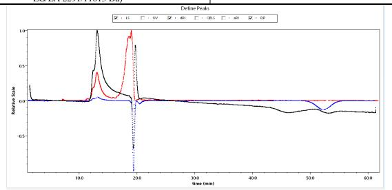
GPC Analysis Method: Agilent 1260 Infinity II HPLC connected to Dawn Heleos II (MALLS), Optilab T-rEX (RI detector) and Viscostar III viscometer operated by Astra 7 software. GPC analysis performed with separation by a linear gradient column (Tosoh Bioscience LLC, TSKgel GMHHR-L, 7.8 mm x 30 cm) at 0.6 ml/min flow of Acetone.
