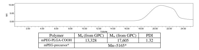
**GPC-ES** Analysis Method: Waters Breeze 2 system with 1 ml/min THF flow across three GPC columns. Detection via refractive index, calibrated against polystyrene standards. \*from MFG data
