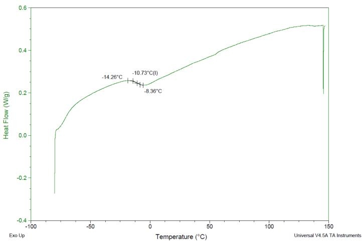
**DSC** Testing: 1-5 mg sample tested in crimped aluminum pan on a TA Instruments Model Q2000 with procedure equilibraion 100 °C, isothermal 5 minutes, equilibrate -80 °C, data on, ramp 10 °C/min to 150 °C. Tg = -10.73 °C
