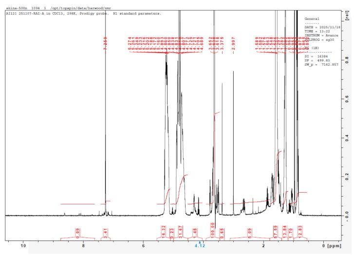
**H-NMR** Spectrum of copolymers in CDCl3 (Bruker  $\geq$ 300 MHz, PINMRF) NMR of PLGA copolymer: EG\*/LA-GA =117\*/76-74 (Mn EG\*/LA:GA 5154\*/5499-4301 Da) LA:GA 56%:44% \*from MFG data
