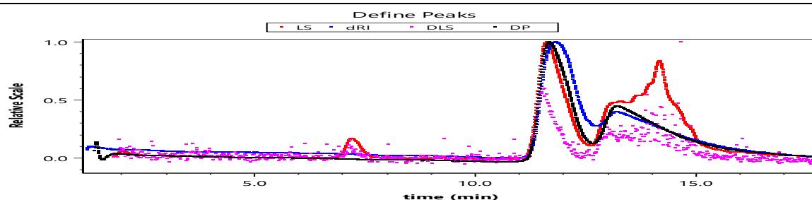
GPC-4D Analysis Method: Agilent 1260 Infinity II system 0.6 ml/min Acetone flow across TSKgel GMHHR-L, 7.8 mm x 30 cm. Detection Dawn Heleos II (MALLS), Optilab T-rex (RI), Dynaprol nanostar (DLS), and Viscostar III (viscosity), universal calibration (Wyatt).
