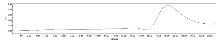
Analysis Method: Waters Breeze 2 system with 1 ml/min DCM flow across three Phenogel 5um columns (Phenomenex). Detection via refractive index, calibrated against polystyrene standards.
