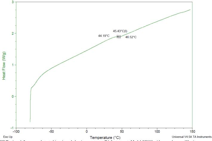
**DSC** Testing: 1-5 mg sample tested in crimped aluminum pan on a TA Instruments Model Q2000 with procedure equilibraion 100 °C, isothermal 5 minutes, equilibrate -80 °C, data on, ramp 10 °C/min to 150 °C. Tg = 45.43 °C
