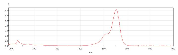
Analysis method: Scan from 190-900nm in 1nm increments of 0.25 mg/mL PLGA-CY5 solution in DCM against DCM blank. Testing of absorbance at 653 nm as compared to a series of CY5 standards has indicated a dye content of  $200.56 \,\mu\text{g/mL}$ .
