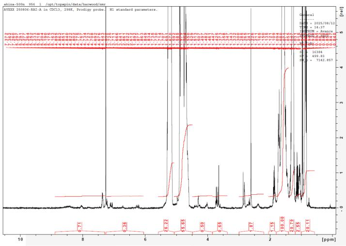
**H-NMR** Spectrum of copolymers in CDCl3 (Bruker ≥300 MHz, PINMRF) NMR of PLGA-CY5 copolymer: LA-GA =49%-51% molar ratio (LA:GA 54%:46%w:w)
