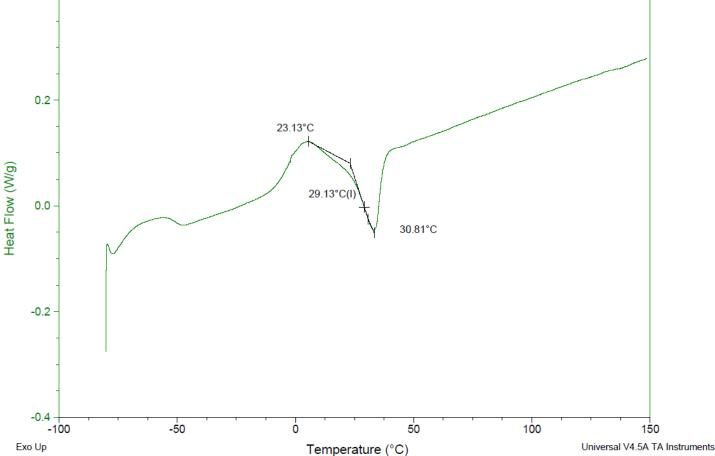
**DSC** Testing: 1-5 mg sample tested in crimped aluminum pan on a TA Instruments Model Q2000 with procedure equilibraion 100 °C, isothermal 5 minutes, equilibrate -80 °C, data on, ramp 10 °C/min to 150 °C. Tg = 29.13 °C
