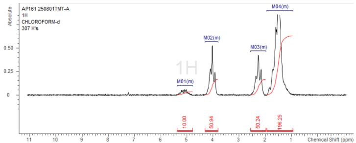
**H-NMR** Spectrum of copolymers in CDCl3 (NMReady-60e, Nanalysis 60 MHz) NMR of PLLCL copolymer: LA-CL =28%-72% molar ratio (LA:CL 20%:80% w:w)
