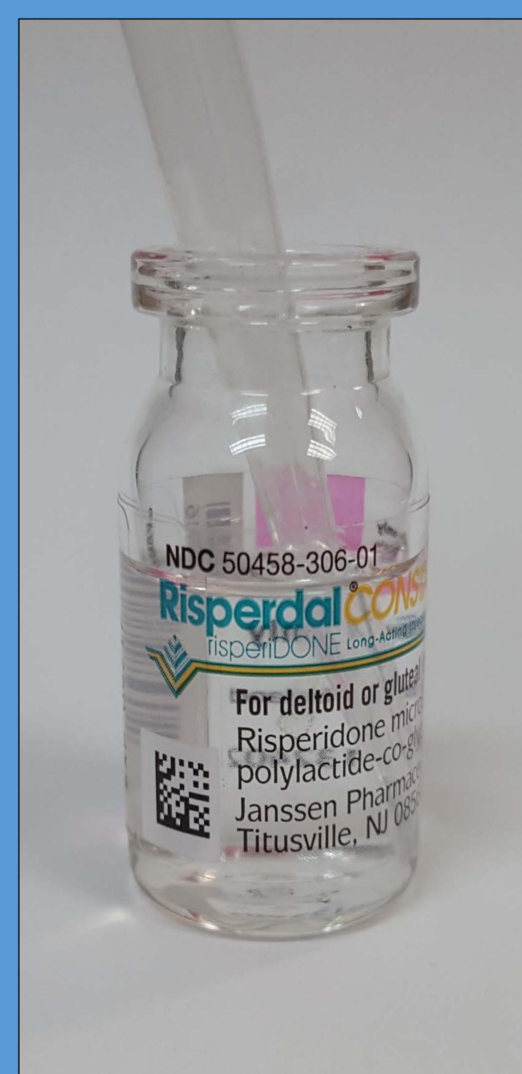
Fig. 1. Dissolution of PLGA microparticles with DCM.
