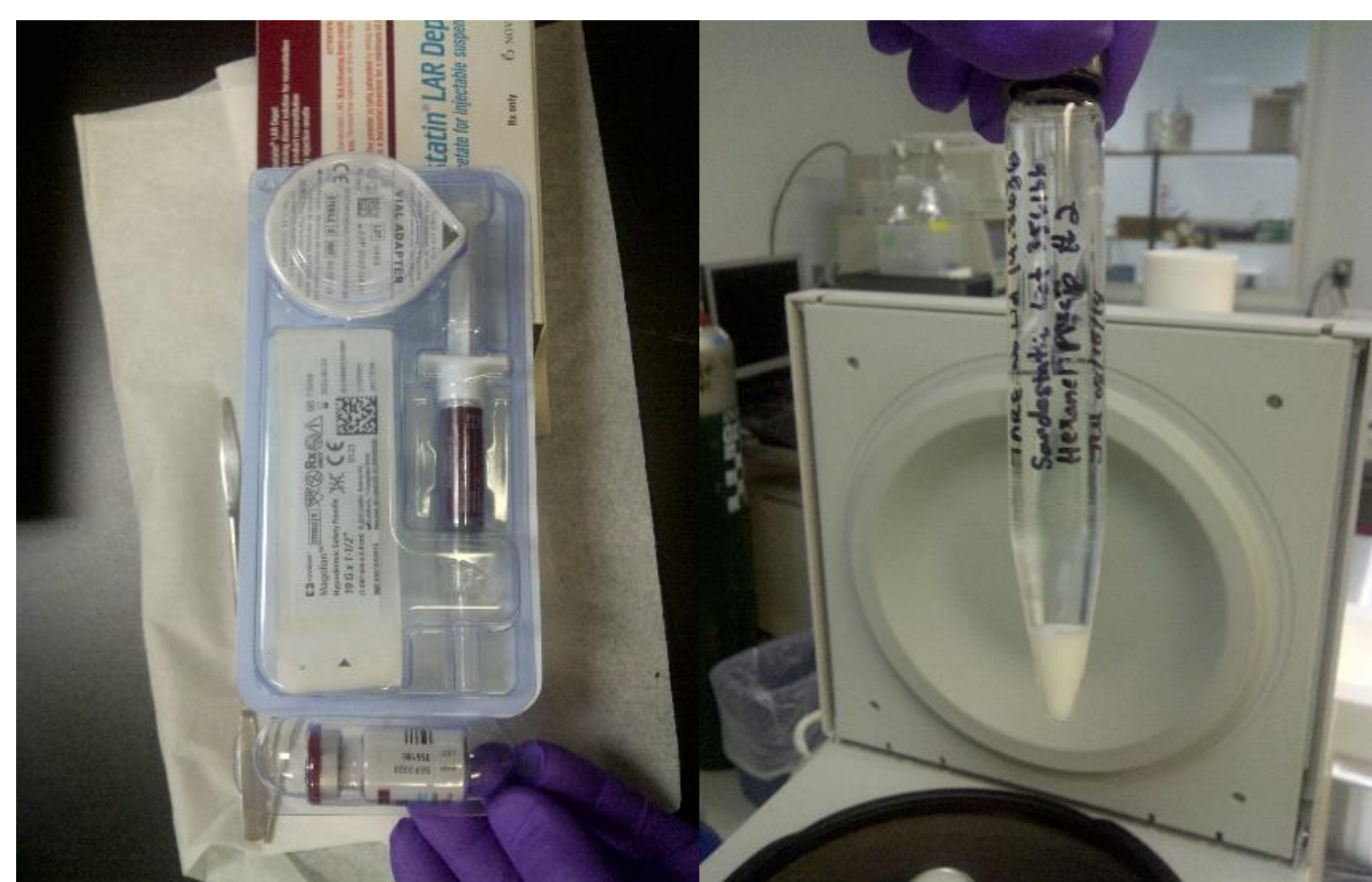
Figure 1. Images from Sandostatin LAR® extraction process. Sample showing vial of material used to extract PLGA and hexane precipitated PLGA extract after centrifugation.
